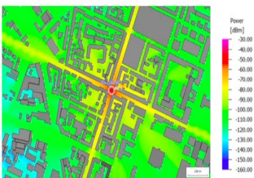
FIGURE 2.1: Received Power heatmap from Winprop
